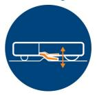
The robot vacuum cleaner comes with a movable nozzle that follows the contours of the floors, carpets, rugs, etc. to ensure accurate cleaning results.
