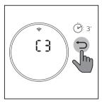
if you don't have the second filter, just tap and hold for 3 seconds to confirm the filter code and exist the filter type change mode.
