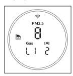
3 Touch and hold the 0 button for 3 seconds to switch off the air purifier.
