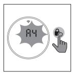
3 Touch and hold → for 3 seconds to confirm the filter code of the new filter.
