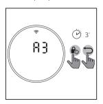
2 Touch and hold for 3 seconds to force reset the filter lifetime counter.
