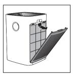
**3** Press the two clips down and pull the pre-filter towards you.
