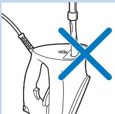
Do not pour water, vinegar, descaling agents or other chemicals into the iron from the opening of the Quick Calc Release.
