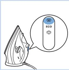
**2** Make sure the steam slider is set to dry setting.
