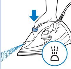
You can use the spray function at any temperature to moisten the garments to be ironed. This helps remove the stubborn creases.
