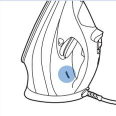
▶ The temperature indicator light goes on while the iron is heating up.
