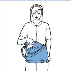
**9** Specific types only: Carry the steam generator by holding it by the handle of the iron with one hand and supporting the bottom with the other hand.
