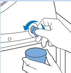
5 Hold a cup under the EASY DE-CALC knob and turn the knob anti-clockwise.
