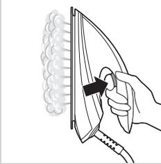
You can use the steam iron in vertical position to remove wrinkles from hanging fabrics.
