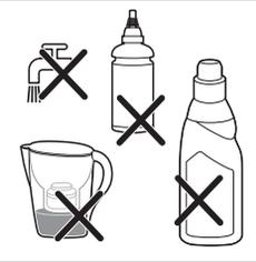
**Caution:** Do not use tap water, perfumed water, boiled water, water from a tumble dryer, rainwater, vinegar, mineral water, magnetically treated water (Aqua+), water from a drinking water filter, starch, descaling agents, ironing aids, salt or chemicals in the water tank. These types of water have been tested. They are not suitable and may even cause damage to the appliance. If you use any of these types of water, your guarantee becomes invalid.
