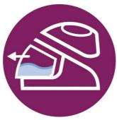
The water tank can be removed to be refilled easily under the tap. The large filling hole makes refilling fast. Thanks to the 1.1-I water tank capacity, you can iron for up to 2 hours continuously without any refile.
