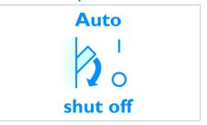
The electronic safety shut-off automatically switches the iron off when it is left unattended or tips over.
