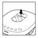
Press the hooks on the top of the steam valve to disassemble it.
