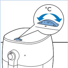
**7** Turn the temperature control knob to the required temperature.
