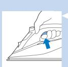
A steam boost from the soleplate helps removing stubborn creases. The steam boost enhances the distribution of steam into every part of the garment.
