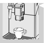
Place a cup under the dispensing spout. Press the " $\bigcup_{MEMO}$ " button to brew an espresso.
