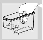
1 Remove the small white filter from the water tank and store it in a dry place.
