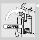
2 Push the lever upwards to select the "COFFEE" function.
