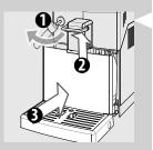
4 Insert the coffee grounds drawer back into the drip tray and place the drip tray back into the machine.
