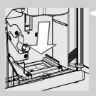
14 Insert the coffee residues drawer in its seat and ensure that it is correctly in place.
