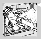
4 To remove the brew group, press the «PUSH» button and pull it by the handle. Pull it out horizontally without turning it.
