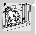
13 After rinsing the brew group, insert it back into its seat until it locks into place (see the "Weekly Cleaning of the Brew Group" chapter). Insert the drip tray and the coffee grounds drawer. Close the service door.
