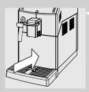
16 Insert the coffee grounds drawer with the drip tray back into the machine and close the service door.
