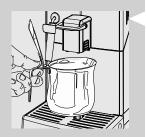
During this process you activate the coffee brewing cycle and fresh water flows through the steam/hot water circuit. This takes a few minutes.
