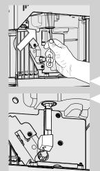
5 Thoroughly clean the coffee duct outlet with the special cleaning tool supplied with the machine or with a spoon handle. Make sure that the cleaning tool is inserted as shown in the figure.
