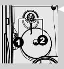
4 The reference marks inside the coffee bean hopper indicate the grind setting. There are 5 different grind settings to choose from, from position 1 (●) for coarse grind - lighter taste to position 2 (•) for fine grind stronger taste. If coffee is watery or is brewed slowly, change the coffee grinder settings.
