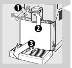
To clean the drip tray, place a "Coffee Oil Remover" tablet inside and fill it 2/3rds full with hot water. Let the cleaning solution take effect for about 30 minutes, then rinse thoroughly.
