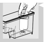
22 Remove the small white filter and replace the INTENZA+ water filter (if installed) in the water tank. Rinse it and fill it with fresh water up to the MAX level. Put it back into the machine.
