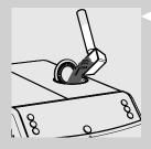
3 Lift the pre-ground coffee compartment lid and add one level measuring scoop of pre-ground coffee. Use only the measuring scoop supplied with the machine. Then close the pre-ground coffee compartment lid.
