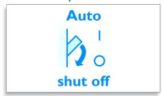
The electronic safety shut-off automatically switches the iron off when it is left unattended or tips over.
