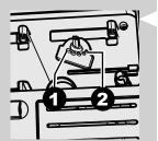
3 The reference marks in the compartment for the coffee bean hopper indicate the grind setting. There are 5 different grind settings to choose from position1 for coarse grind - lighter taste to position 2 for fine grind - bolder taste.
