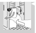
**5** Push gently on the edge of the water tank door to release the hand-grip.
