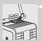
2 Lift the pre-ground coffee compartment lid and add one scoop of pre-ground coffee to the compartment. Use only the measuring scoop supplied with the machine. Then close the pre-ground coffee compartment lid.
