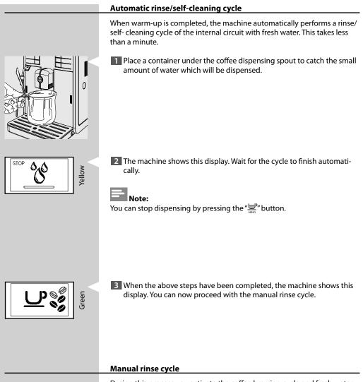
During this process you activate the coffee brewing cycle and fresh water flows through the water circuit. This takes a few minutes.
