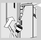
27 Insert the Automatic Milk Frother until it locks in place on the rubber grip.
