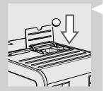
**3** Put a "Coffee Oil Remover" tablet in the pre-ground coffee compartment.
