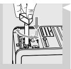
2 Press and turn the grinder adjustment knob under the coffee bean hopper one notch at a time. Use the coffee grinder adjustment key provided with the machine. You will taste the difference after brewing 2-3 cups of coffee.
