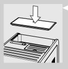
**3** After removal put the protection cover on the machine to prevent dust.
