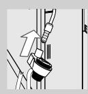
2 Insert the Automatic Milk Frother until it locks in place in the steam wand seat.
