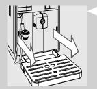
**3** Remove the drip tray. Empty and clean the drip tray:
