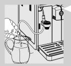
3 Insert the suction tube in the milk container.
