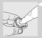
**23** Reassemble the lid. Make sure that you press it in the middle to have it correctly inserted.
