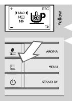
5 When the display value is changed, the "OK" message appears. Press the "₩" MENU button to confirm the change.
