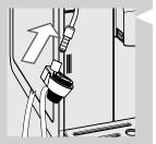
26 Remove the small white water filter and place back the "INTENZA+" water filter into the water tank if it was installed and the Automatic Milk Frother.
