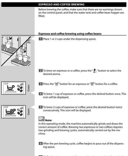
7 Coffee brewing automatically stops when the preset level is reached; press the """ button to stop it earlier.
