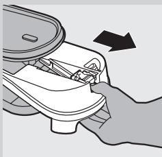
Never remove the Calc-Clean rinsing cap when the steam generator is hot.
