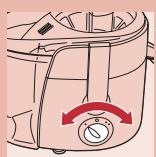
**3** Switch the appliance on by turning the control knob to setting 1 (low speed) or 2 (normal speed).
