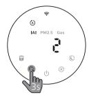
With the light sensor, the control panel can automatically turn on, turn off or dim according to the ambient light. The control panel will be off or dim when the ambient light is dark. You can touch any button to wake up all lights. Then, if no further operation, all lights will be off or dim again to match with the ambient light.
