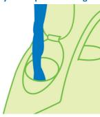
the huge filling hole, and the sideways opening door of the Philips iron.
