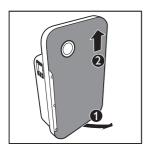
3 To remove the pre-filter, grab the two projections and pull the filter towards you.
