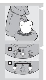
3 Put a bowl (with a capacity of at least 1500ml) under the coffee spout to collect the water.
