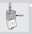
2 Fill the water reservoir with cold water up to the **MAX** indication and put it back onto the machine.
