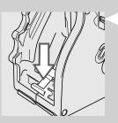
Gently pull down the lever until it is in contact with the brew group base and the two reference signs on the side of the brew group do match.
