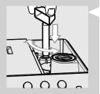
1 'Press and turn the grinder adjustment knob below the coffee bean hopper one notch at a time. Use the coffee grinder adjustment key provided with the machine.' You will taste the difference after brewing 2-3 cups of coffee.
