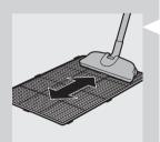
3 Clean the pre-filter by removing the dust with a vacuum cleaner.
