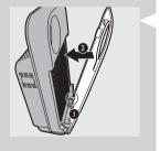
To reattach the front panel, insert the bottom hooks into the bottom of the appliance first (1). Then push the panel against the body of the appliance (2).
