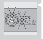
■ The power-on light, the AUTO light, and the AIR QUALITY light on the control panel go on.
