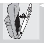
To reattach the front panel, insert the bottom hooks into the bottom of the appliance first (1). Then push the panel against the body of the appliance (2).
