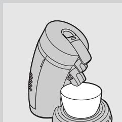
**5** Put a bowl with a capacity of at least 1.6 qt./1.5 litres under the spout to collect the descaling mixture.
