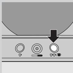
**6** Press the 2-cup button
