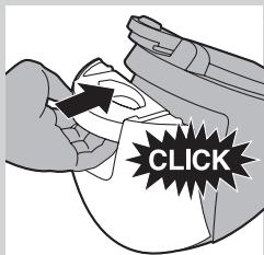
**3 Slide the water tank back into the steam generator ('click').**
