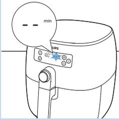
**8** After the temperature is confirmed, the time indication “- -” starts blinking.
