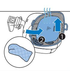
4 Carefully remove the splatter-proof lid.
