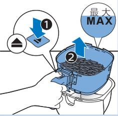
**13** Press the basket release button and lift the basket out of the pan.
