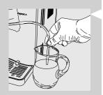
5 Remove the suction tube from the tube holder and put it into the milk container.
