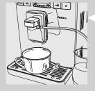
1 Insert the suction tube in the milk container. Place a cup under the Cappuccinatore.
