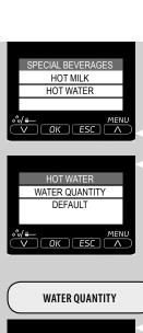
2 Select HOT WATER by pressing the "√" or "∧" scrolling button. Press "OK" to confirm.
