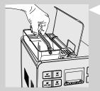
7 Open the lid and remove the water tank by the handle.
