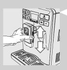
The height of the dispensing spout can be adjusted to better fit the dimensions of the cups that you wish to use.
