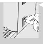
5 Fit the Cappuccinatore suction tube holder into the first lower slot of the machine.
