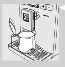
18 Place a container under the dispensing spout to catch the small amount of water which will be dispensed.
