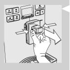
1 Press the side buttons to remove the water dispenser (if installed).
