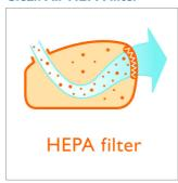
The High Efficiency Particulate Air filter filters fine dust from the air. This guarantees more dust is captured.
