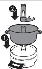
1 Put the pot on the base (1) and put the stirrer on the spindle (2).
