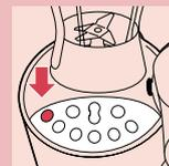
**6** Press the blending process button. The blender will start to operate, the speed increases to maximum speed and will continue to run at this speed until the STOP button is pressed. During the blending process the speed can be decreased up to three times by pressing the - button.
