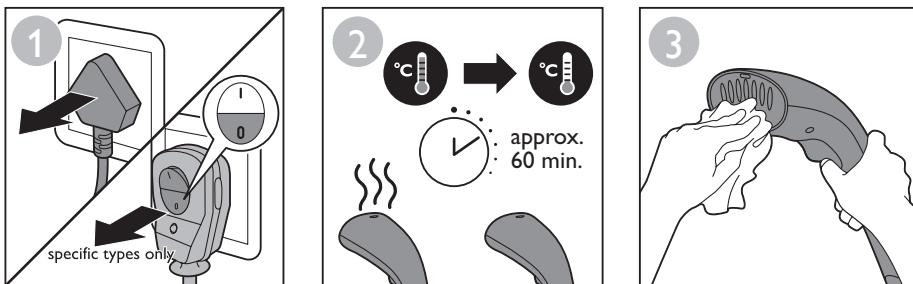
**EN** Clean the appliance and wipe any deposits off the steamer head with a damp cloth and a non-abrasive liquid cleaning agent.
