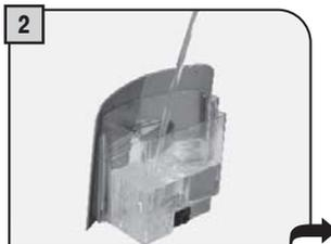
Empty the tank and refill it, dissolving the descaling solution into a full tank of water.
