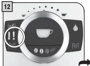
At the end of the rinse cycle, the descaling light will turn off and the warning light will turn on. The descaling cycle is complete.
