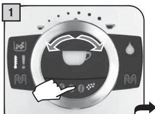
Adjust the quantity of coffee to be brewed by turning the knob. Press the aroma button until the pre-ground icon is illuminated.
