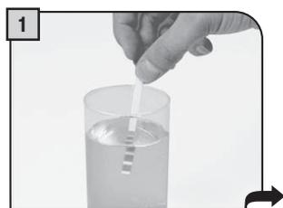
Immerse the water hardness test strip provided with the machine in water for 1 second.
