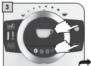
Simultaneously press and hold for 3 seconds to access the programming mode.
