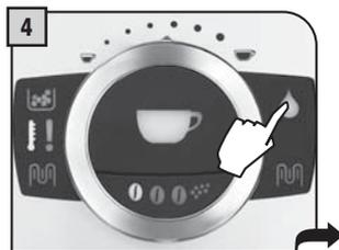
Press the water button until the water hardness value is reached.
