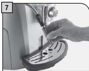
When the wand has cooled down, disassemble it and wash it carefully.
