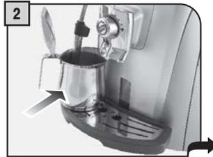
Place a container beneath the hot water wand.
