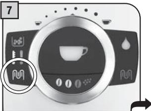
During the descaling and rinse cycle the light is constantly on. Empty the container if it becomes too full.
