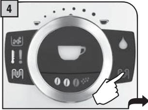
Press the descaling button for 5 seconds.
