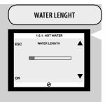
By adjusting the bar on the display by pressing the " $\nabla$ " or " $\Delta$ " scrolling button, you can choose the quantity of hot water to be dispensed. Press "**OK**" to confirm the adjustment.
