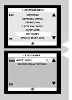
1 Select "HOT WATER" from the beverage menu by pressing the "▼" or "▲" scrolling button. Press "**OK**" to confirm.
