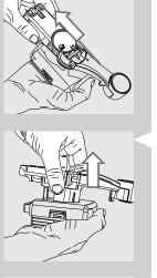
5 Remove the connector which is in contact with the machine.
