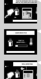
10 Press the "OK" button to start the cycle. The machine starts dispensing the cleaning solution through the milk dispenser.
