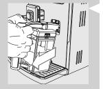
**3** Pull away from the machine until it is completely detached.
