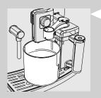
Place a large container (1,5 lt ) under coffee the dispensing spout. Open the milk dispenser by turning it clockwise.
