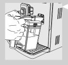
2 At this stage the carafe holes (A) are lower than the couplings (C). The pins (B) are located at the same height of the guides (D).
