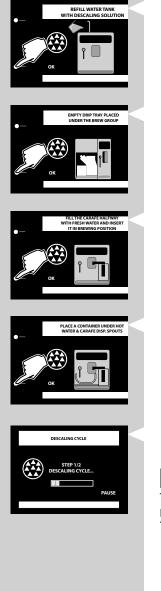
4 Remove the water tank, and if installed, remove the INTENZA+ water filter. Pour the entire content of the Saeco decalcifier. Then fill the water tank with fresh water up to the MAX level. Press the "**OK**" button.
