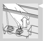
1 Remove the small white filter from the water tank and store it in a dry place.
