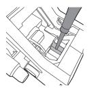
3 Apply a thin layer of grease around the shaft in the bottom of the brew group.
