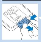
The remote control works on a CR2025 coin-shaped battery. Replace the battery when the robot no longer responds when you press the buttons on the remote control.
