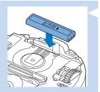
4 Place the rechargeable battery into the battery cavity.
