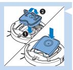
6 Put the dust container back into the dust container compartment and put the top cover back onto the robot.
