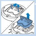
2 Pull up the handle of the dust container lid and lift the dust container out of the dust container compartment.
