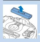
Replace the rechargeable battery when you can no longer recharge it or when it runs out of power quickly. You can order a new rechargeable battery under order number CP0113 for FC8820 and order number CP0112 for FC8810.
