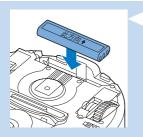
3 Place the new rechargeable battery in the battery cavity and slide the battery cavity cover back onto the robot.
