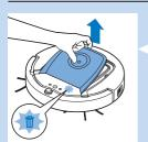
Empty and clean the dust container when the dust container full icon on the display of the robot lights up.
