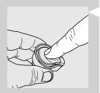
**22** Attach the lid by pressing in the middle and ensure that it is firmly in place.
