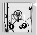
4 The reference marks inside the coffee bean hopper indicate the grind setting. There are 5 different grind settings to choose from, from position 1 (●) for coarse grind - lighter taste to position 2 (•) for fine grind - stronger taste. If coffee is watery or is brewed slowly, change the coffee grinder settings.
