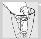
2 Remove the "INTENZA+" water filter from its packaging, immerse it vertically (with the opening positioned upwards) in cold water and gently press the sides so as to let the air bubbles out.
