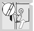
**26** Put the components back onto the steam wand.
