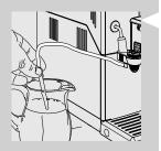
6 Insert the suction tube into the milk container.
