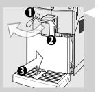
4 Insert the coffee grounds drawer back into the drip tray and place the drip tray back into the machine.
