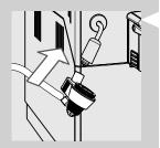
4 Insert the Automatic Milk Frother into the steam wand seat.
