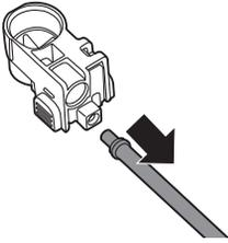
5 Remove the tube with the fitting.
