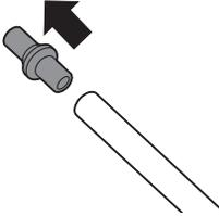
6 Remove the fitting from the tube.
