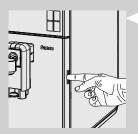
4 Press the button in the frame and open the service door.
