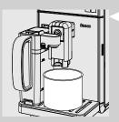
2 Pull out the carafe dispensing spout to the right up to the "O" icon. Place a container under the carafe dispensing spout.
