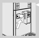
7 Check that the water dispensing spout is correctly installed.
