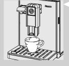
2 Press and hold the Espresso " button until the "MEMO" icon appears on the display, then release the button. The machine is now in programming mode. The machine starts brewing coffee.
