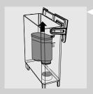
6 Remove the water tank and empty it. Remove the AquaClean filter.
