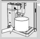
10 Place a large container (1.5 l) under both the milk carafe dispensing spout and the coffee dispensing spout. Press the "\square" button to confirm.
