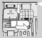
Insert the carafe into the machine. Slide the carafe dispensing spout to the right up to the "O" icon. Press the "√" button to confirm.
