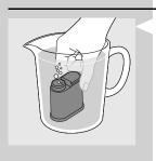
1 Remove the AquaClean filter from its packaging, shake it for 5 seconds and immerse it vertically (with the opening positioned upwards) in cold water, delicately pressing the sides so as to let the air bubbles out.
