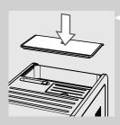
3 After removing it, put the protection cover (if any) on the machine to keep it dust-free.
