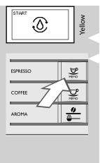
2 Press the " $\frac{-p}{NBHO}$ " button to start the circuit priming cycle.
