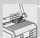
2 Lift the pre-ground coffee compartment lid and add one level measuring scoop of pre-ground coffee. Use only the measuring scoop supplied with the machine. Then close the pre-ground coffee compartment lid.
