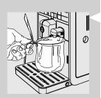
During this process, fresh water flows through the internal circuit of the machine and the machine warms up. This takes a few minutes.
