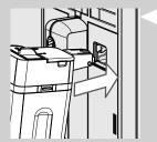
2 Slightly tilt the milk carafe. Insert it all the way into the guides of the machine.
