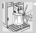
During this process you activate the coffee brewing cycle and fresh water flows through the water circuit. This takes a few minutes.
