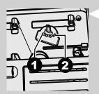
3 The reference marks in the coffee bean hopper compartment indicate the grind setting. There are 5 different grind settings to choose from, from position 1 for coarse grind - lighter taste to position 2 for fine grind - stronger taste. If coffee is watery or is brewed slowly, change the coffee grinder settings.
