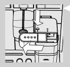
Insert the carafe into the machine. Pull out the milk carafe dispenser to the left up to the " — " icon.
