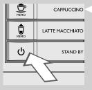
3 If the cycle was interrupted during the descaling phase, it will be resumed from step 12 of the "Descaling" chapter. Press the "♥" button to restart the cycle.
