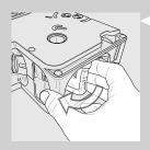
12 Turn the brew group back to the off position by manually turning the pin on the base, as shown in this figure. Turn it until it locks into the position described in the following step.
