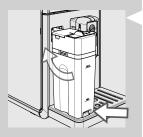
Push the carafe towards the bottom while rotating at the same time, until it is locked at the drip tray.
