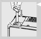
1 Press and turn the grinder adjustment knob inside the coffee bean hopper **one notch at a time**. Use the coffee grinder adjustment key provided with the machine. You will taste the difference after brewing 2-3 cups of coffee.
