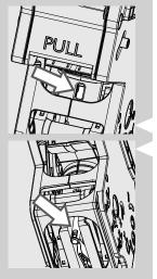
2 Lubricate also the piston, as shown in the figure.
