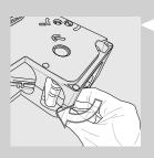
13 When you reach the position shown in this figure, check that the two reference signs match and that the brew group is locked into position.
