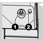
2 The reference marks in the coffee bean hopper compartment indicate the grind setting. There are 5 different grind settings to choose from position 1 for coarse grind - lighter taste to position 2 for fine grind - bolder taste.
