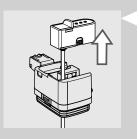
3 Lift the dispensing spout to remove it from the top of the carafe. The milk carafe dispenser is made up of five parts that must be disassembled. Each part is indicated by a capital letter (A, B, C, D, E) as shown in the figure below.
