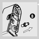
**5** Remove the fitting (B) from the milk frother by pulling it outwards.
