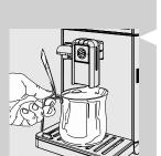
You need to perform a rinse cycle when using the machine for the first time. During this process, the coffee brewing cycle is activated and fresh water flows through the dispensing spout. This takes a few minutes.
