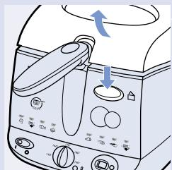
**8** Open the lid by pressing the release button. The lid will open automatically.
