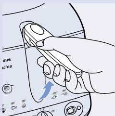
**1** Lift the handle to raise the basket to its highest position, the 'drip-out position'.
