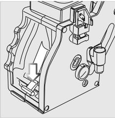
**8** Gently pull down the lever until it is in contact with the brew group base and the two reference signs on the side of the brew group do match.
