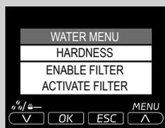
**7** Select HARDNESS option by pressing the "OK" button and set the water hardness value.
