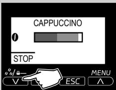
8 Once the milk froth has been poured, the machine brews coffee. The brewing can be stopped earlier by pressing the "V" button.
