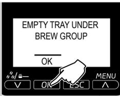
**10** Empty the (internal) drip tray and place it back. Then, press the “OK” button.
