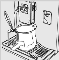
6 Place a container (1,5 Lt) under the coffee dispensing spout. Press the "OK" button to start the cleaning cycle.
