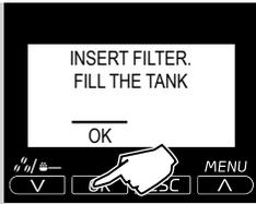
**12** Press the “OK” button to confirm that you have inserted the water filter and filled the water tank.
