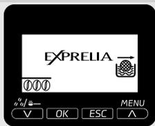
When the “INTENZA+” water filter needs to be replaced with a new one, this icon is displayed “
