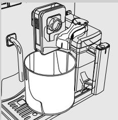
**15** Empty the container and place it back under the coffee dispensing spout. Open the milk dispenser by turning it clockwise.
