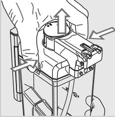
**2** Press the release buttons to allow the lid removal.
