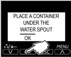
**13** Press the “OK” button to confirm that a container is placed under the water spout.
