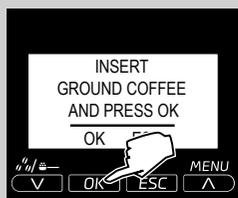
4 Press the “OK” button. The machine starts dispensing water.
