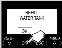
4 Fill the water tank with fresh water up to the MAX level. Press the "OK" button.
