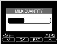
By adjusting the bar on the display by pressing the “V” or “^” scrolling button, you can choose the quantity of milk to be used for the selected beverage. Press OK to confirm the adjustment.
