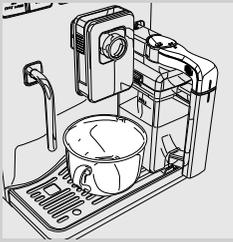
**2** Place a cup under the dispensing spout and open the milk carafe dispenser by turning it clockwise.
