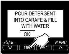
**10** Press the "OK" button to start the cycle. The machine starts dispensing the cleaning solution through the milk dispenser.
