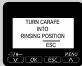
Close the milk dispenser of the carafe to start the rinsing cycle of the carafe. Press the button "ESC" to exit.
