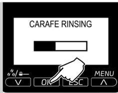
**16** The machine starts dispensing water from both the coffee and the milk dispenser. The bar shows the cycle progress.
