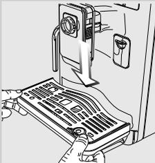
**5** Dry, reassemble and reinsert it in the machine.
