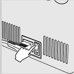
**12** Switch the power button to "I" to turn on the machine.
