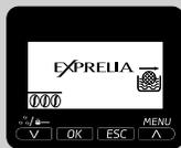
The machine needs the "INTENZA+" water filter to be replaced.
