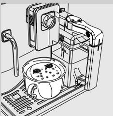
9 Remove the cup and close the milk dispenser by turning it counter clockwise.
