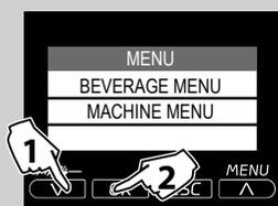
**5** Press the "V" button to scroll down the pages. Press "OK" to select MACHINE MENU.
