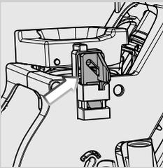
**9** Make sure the hook to lock the brew group is in the correct position by firmly pressing the "PUSH" button until you hear a click. Check if the hook is at the top end position. If it is not, please try again.
