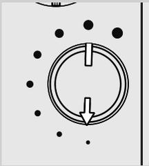
When you adjust the ceramic coffee grinder to a finer setting, your coffee will taste stronger. For a milder coffee taste, adjust the ceramic coffee grinder to a coarser setting.
