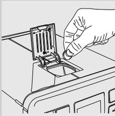
5 Put a "Coffee Oil Remover" tablet in the pre-ground coffee compartment. Press the "OK" button.
