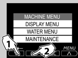
**9** Press the "V" button to select WATER MENU. Press "OK" to confirm.
