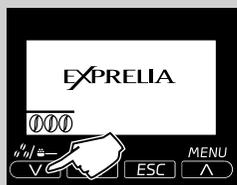
**1** To temporarily change the amount of coffee ground, press the "V" button on the control panel.
