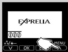
**4** Now you can program the water hardness setting. Press "MENU" button to access the machine main menu.
