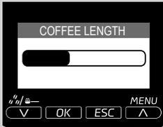
By adjusting the bar on the display by pressing the “V” or “^” scrolling button, you can choose the quantity of water used for coffee brewing. Press OK to confirm the adjustment.
