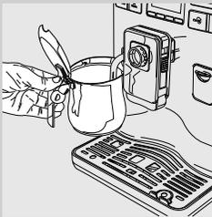
1 Place a container with the desired product you want to heat under the hot water/steam wand.
