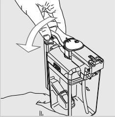
**7** Rotate the milk dispenser counter-clockwise to the lock position.
