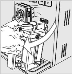
**13** Remove the milk carafe and the container from the machine.
