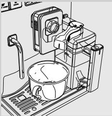
1 Insert the milk carafe and place the cup under the dispensing spout. Open the milk dispenser by turning it clockwise.
