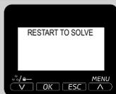
Take note of the code (E xx) shown in the display at the bottom. Turn off the machine. After 30 seconds, turn it on again. Try this 2 or 3 times. If the machine does not start, contact the Philips SAECO hotline in your country and tell them the code shown in the display. You can find its contact details in the warranty booklet by-packed separately or on [www.philips.com/support](http://www.philips.com/support).
