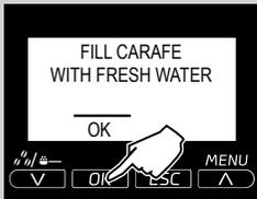
**14** Wash the milk carafe thoroughly and fill it with fresh water. Insert the milk carafe into the machine. Press the "OK" button to confirm.
