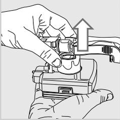
**6** Remove the handle with the suction tube.
