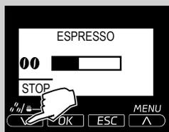
**6** Coffee brewing stops automatically when the pre-programmed level is reached; it is possible to stop earlier by pressing "✓" button.
