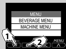
**7** Press the "MENU" button to access the machine main menu.
