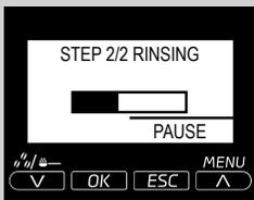
**13** The rinsing cycle is activated. The bar shows the cycle progress.
