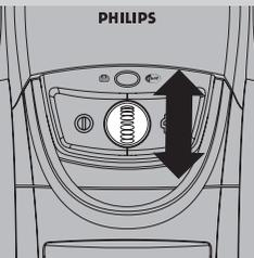
During vacuuming, you can adjust the suction power with the selection wheel on top of the appliance.
