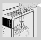
3 Thoroughly clean the pre-ground coffee compartment with the cleaning brush, making sure that there are no more coffee residues in the duct.
