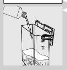
6 Remove the water tank and the "INTENZA+" water filter (if installed) and insert the small white filter supplied with the machine. Pour the entire content of the Saeco descaling solution.
