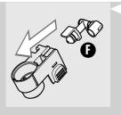
10 Insert the fitting (F) into the milk frothing device by pressing it up to its limit.
