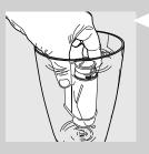
1 Remove the "INTENZA+" water filter from its packaging, immerse it vertically (with the opening positioned upwards) in cold water and gently press the sides so as to let the air bubbles out.
