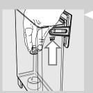
10 Remove the small white filter from the water tank and store it in a dry place.
