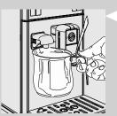
6 Dispense the desired amount of hot water. To stop the hot water dispensing, press the Special Beverages " button again.
