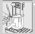
9 Place a container (1.5 l) under the coffee dispensing spout. Press the "\sqrt{"}" button to start the cleaning cycle.
