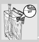
15 At the end, fill the water tank again up to the MAX level. Now the machine is ready to brew coffee. This icon will be displayed.
