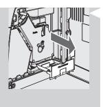
2 Empty and clean the coffee residues drawer located in side of the machine. Open the service door, remove the drawer and empty the coffee residues.
