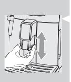
The height of the dispensing spout can be adjusted to better fit the dimensions of the cups that you wish to use.
