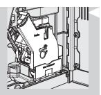
11 After rinsing the brew Group, insert it again in its seat until it locks into place (see "Weekly cleaning of the brew group" chapter). Insert the coffee residues drawer and the coffee ground drawer. Close the service door.
