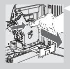
9 Remove the coffee ground drawer and open the service door. Remove the coffee residues drawer and then the brew group.
