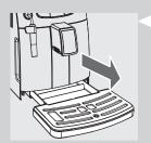
15 To clean the drip tray, place a "Coffee Oil Remover" tablet inside and fill it up to 2/3rds full with hot water. Let the cleaning solution take effect for about 30 minutes, then rinse thoroughly.
