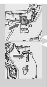
10 Make sure the hook to lock the brew group is in the correct position by firmly pressing the "PUSH" button until you hear a click. Check if the hook is at the top end position. If it is not, please try again.
