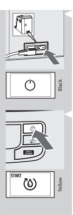
12 Switch the power button to "I" to turn on the machine. The display shows the stand-by icon.
