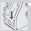
Gently pull down the lever until it is in contact with the brew group base and the two reference signs on the side of the brew group do match.
