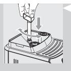
1 Press and turn the grinder adjustment knob one notch at a time. You will taste the difference after brewing 2-3 cups of espresso.
