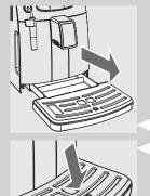
3 Empty and clean the drip tray. Perform this operation also when the full drip tray indicator is raised.
