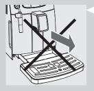
NEVER remove the drip tray when the machine has just been turned on. Wait a couple of minutes, since the machine will carry out a rinse/ self-cleaning cycle.
