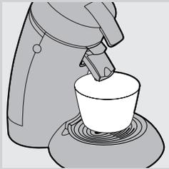
**8** Put a bowl (with a capacity of at least 1500ml) under the coffee spout to collect the water.
