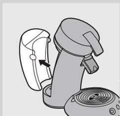
**2** Fill the water reservoir with cold water up to the **MAX** indication and put it back onto the machine.
