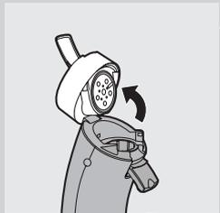
**5** Put the 1-cup pod holder ☺ or the 2-cup pod holder ☺☺ in the machine without pod(s).
