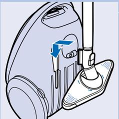
**4** Put the appliance in upright position and attach the nozzle to the appliance by inserting the ridge on the nozzle in the slot.
