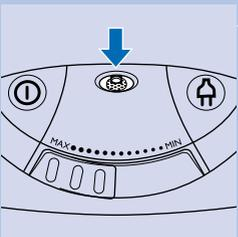
**1** Replace the dustbag as soon as the dustbag-full indicator changes colour (even when the nozzle is not placed on the floor).
