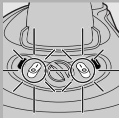
**3** Put the mains plug in an earthed wall socket and set both the steam tank switch and the iron switch to 'on'. The steam tank and the soleplate will now heat up.
