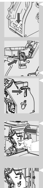
**10** Gently pull down the lever until it is in contact with the brew group base and the two reference signs on the side of the brew group match.
