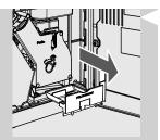
3 Empty and clean the coffee residues drawer located on the side of the machine. Open the service door, remove the drawer and empty the coffee residues.
