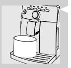
6 Place a large container (1.5 l) under the steam/hot water wand and the dispensing spout.
