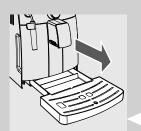
2 Empty and clean the drip tray. Perform this operation also when the full drip tray indicator is raised.
