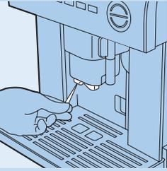
**4** Make sure that the holes in the coffee spout are not blocked. If they are blocked, unblock them by scraping dried coffee residues away with a needle.
