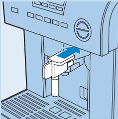
**6** Insert the hot water spout into the appliance.
