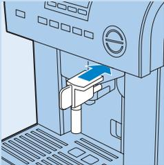
**1** Attach the hot water spout to the nozzle.
