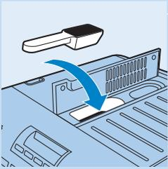
**4** Open the lid of the ground coffee container and put one level measuring spoon of ground coffee in the funnel.
