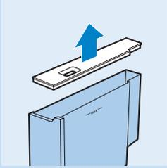
**4** Rinse the water tank and fill it with fresh water. Remove the lid to create a bigger filling opening.
