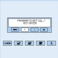
**3** Press the button for hot water until the message 'PROGRAM TO SET VOL. - HOT WATER' appears on the display and then release it.
