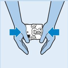
*Note: If you cannot insert the brewing unit, press the unit firmly from above and below at the same time and then try to insert it. If you still cannot insert the brewing unit, close the service door, unplug the appliance and then plug it in again. Wait for all the lights to go off after the self-check, then open the service door and reinsert brewing unit.*
