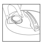
(2) Turn the steam valve to the open position to remove.
