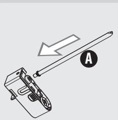
**14** Insert the suction tube with the fitting (A) into the milk frother.
