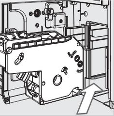
**16** Insert the brew group back into its seat by sliding it along the guides until it locks into place.
