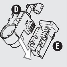
**11** Insert the milk frothing device (D) into the support (E).
