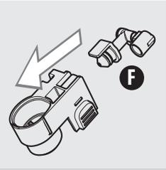
**10** Insert the fitting (F) into the milk frothing device by pressing it up to its limit.
