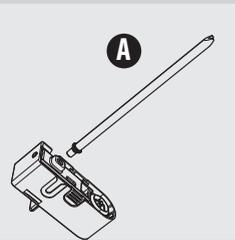
**4** Remove the suction tube with the fitting (A) from the milk frother.
