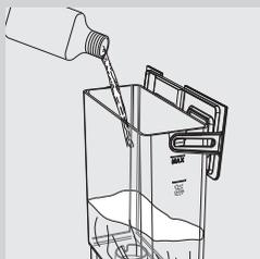
6 Remove the water tank and the "INTENZA+" water filter (if installed) and insert the small white filter supplied with the machine. Pour the entire content of the Saeco descaling solution.
