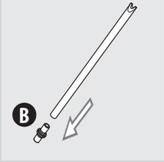
5 Remove the fitting (B) from the suction tube.
