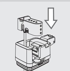
**6** After installing the suction tube with the fitting, insert the carafe dispenser on the top of the carafe.
